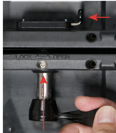
2. Press the spring-loaded locking latch toward the left while pressing the vertical connector upwards into the locking latch.
