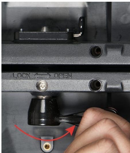
4. To unlock, twist the vertical connector lever to the right, towards the direction marked "OPEN". The locking post will then drop out of place. Press the latch to the left if needed to help release the locking post.
