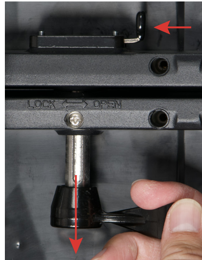
4. To unlock, twist the vertical connector lever to the right, towards the direction marked "OPEN". The locking post will then drop out of place. Press the latch to the left if needed to help release the locking post.
